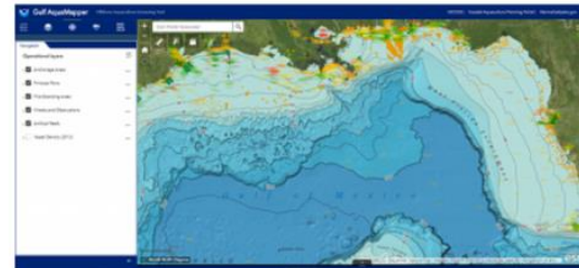
A screenshot of the Gulf Aquamapper tool's online interface, which provides data to help with permitting and siting of potential offshore aquaculture ventures. Credit: NOAA
